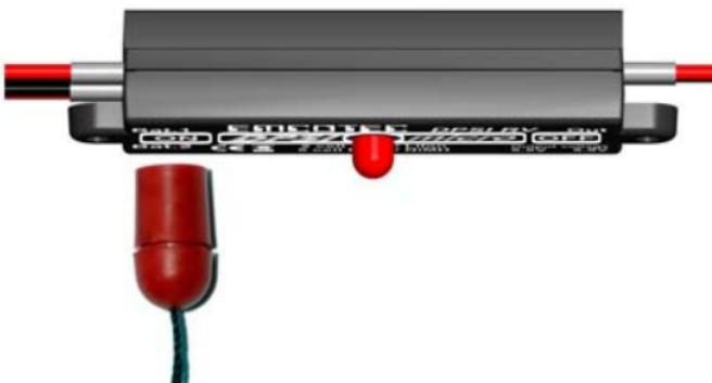
In case one battery is not connected to the **DPSI RV** or one of both batteries is defective, the **DPSI RV** starts in programming mode. This mode is left automatically after approx. 30 seconds. Within these 30 seconds, a missing second battery must not be connected, if reprogramming is not desired.
