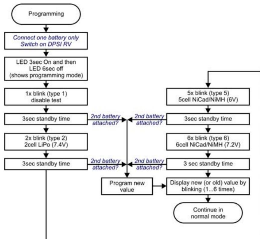
Alternatively programming or programming of a **MPS RV** via sliding switch as described! Because only one battery is used for the **MPS RV**, programming only works by using the voltage selection switch!
